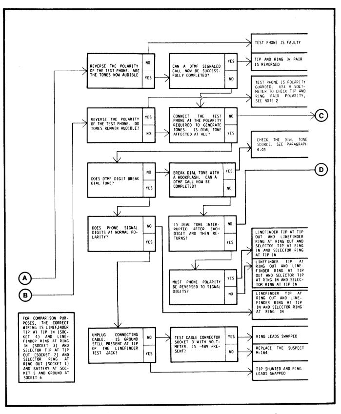
Figure 13 Installation Test Post-Fuse Faults (Sheet 2 of 4)
