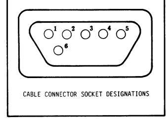
Figure 12 Connector Cable Sockets
