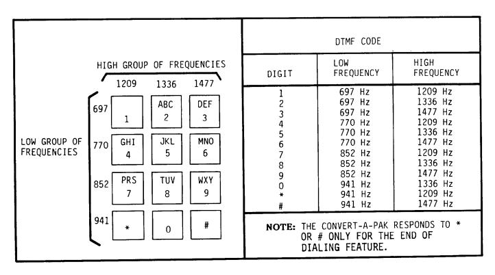
Figure 3 DTMF Digit Buttons and Code
