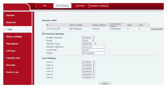
On the SIP Hotspot tab page, set Enable Hotspot to Disabled and then the line registration information of the SIP hotspot client connecting to the hotspot will be cleared. When the telephone set functioning as the SIP hotspot is suspended, the line registration information will not be cleared.
