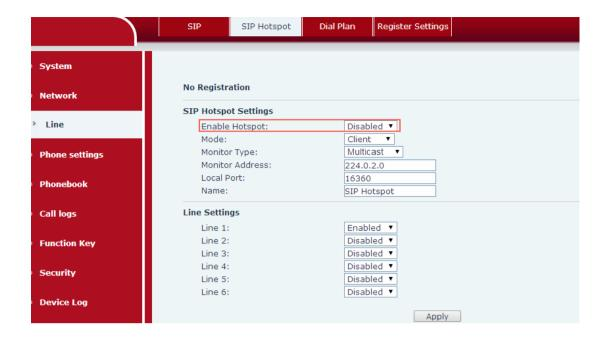
After suspension, the line registration information about the SIP hotspot client will be cleared. See the figure below.
